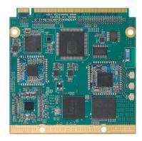
ExSOM-4412 is a full featured **System on Module** that integrates all the core components of a Single Board Computer and can be mounted onto an application specific base board. It has a standardized form factor of 70mm x 70mm and have specified pin outs based on the high speed 230-pin MXM connector and provides the functional requirements for all kinds of embedded applications.
